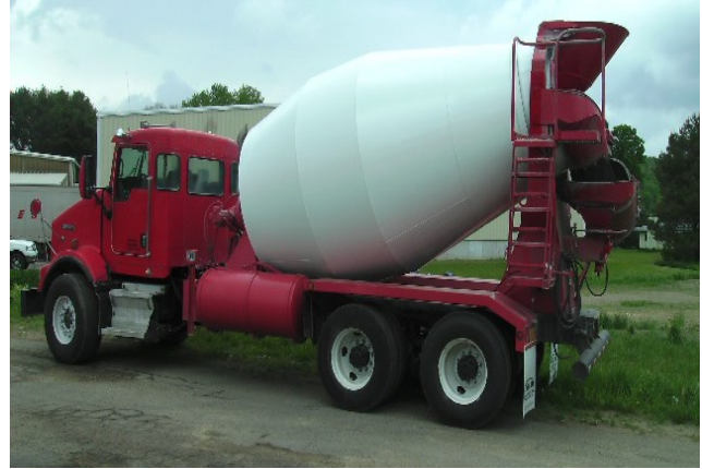
New Drum installed and painted.
