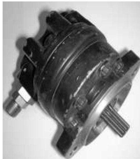
H1040 - Eaton Chute Pump
