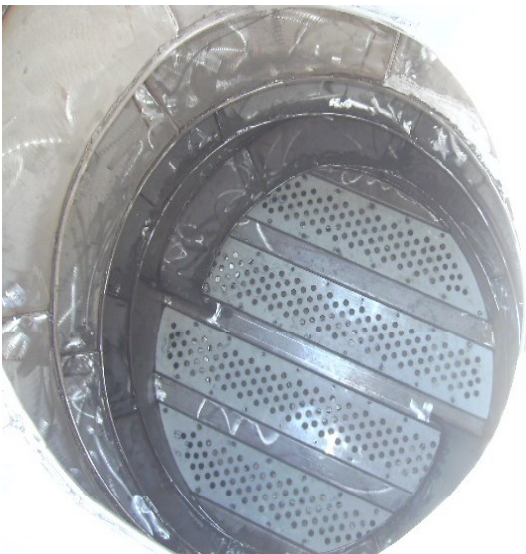
Strainer built into the head of the drum to discharge tanning solution thru 4" valve
