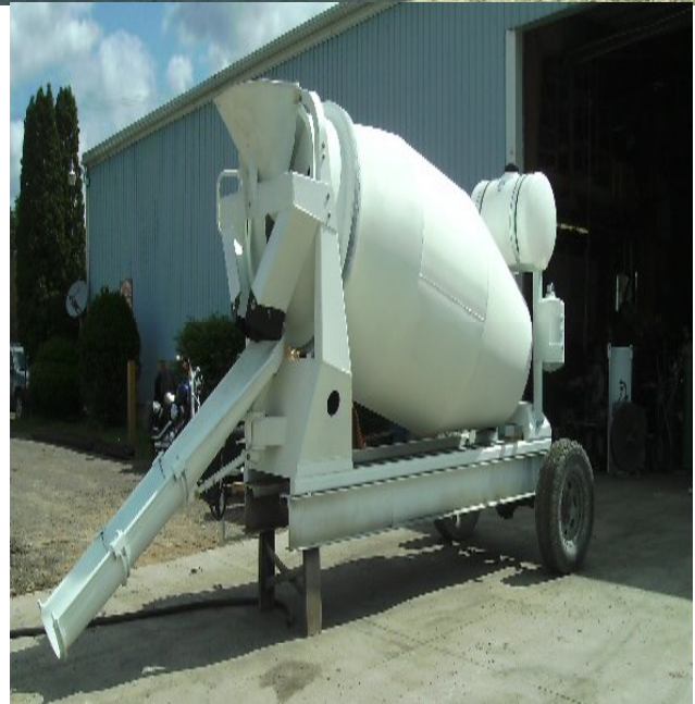
26hp Honda Gas Engine runs mixer
